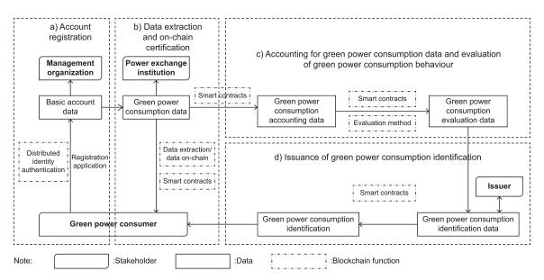
Figure 3—Application model of the blockchain platform for green power identification application
